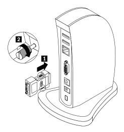
To use the DVI-I to VGA adapter with an external monitor, do the following:
